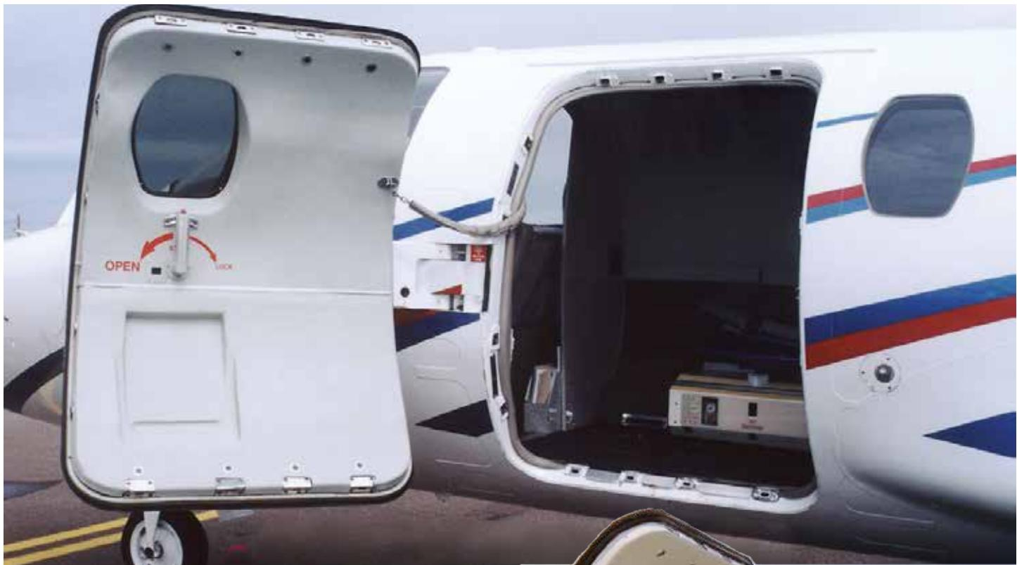
**S**kyWay's extended-width door modification is the perfect solution to outfit your Cessna Citation for air medical or cargo missions. It provides superb cabin access for large, bulky items without compromising the structural integrity of the Citation airframe.
