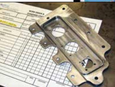
A typical process begins with boring precision holes in a "blank" of high-grade aluminum, steel or other metal.
